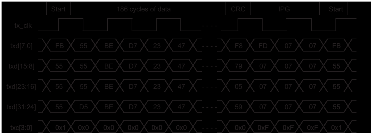
Figure 8. Packet Transmission at the XGMII Interface
