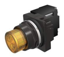
30mm BlackMax, Epoxy Coated Corrosion Resistant Complete Metal Unit Illuminated Indicator Light Transformer type, 480V AC LED Lamp, BA9s Plastic Lens, Amber UL Listed, CSA Certified NEMA 1,3,3R,4,4X,12,13 & Automotive Standards
