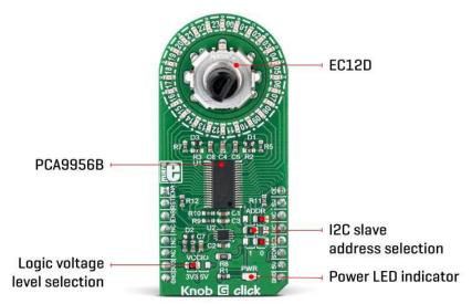
This Click Board uses the EC12D, a 15-pulse incremental rotary encoder with a push-button, from ALPS. This encoder has very good mechanical specifications: debouncing time for its internal switches goes down to 2ms, and it can withstand a huge number of switching cycles, up to 30,000. The supporting debouncing circuitry allows contacts to fully settle before the output is triggered.
