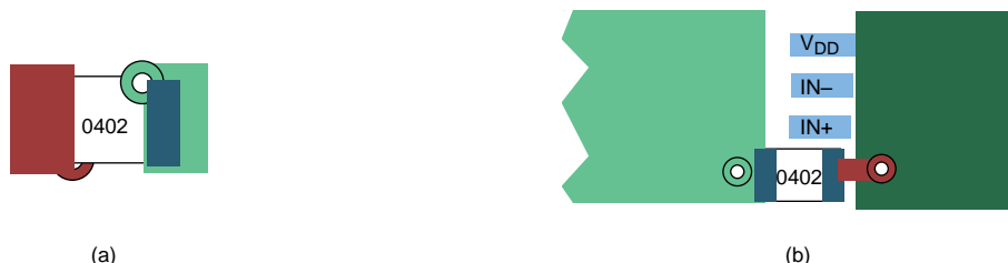
Figure 30. Typical Decoupling Capacitor Layouts
