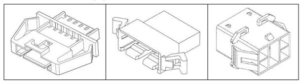
Mounting ears are designed for high panel retention strength within a minimal panel space. Inserting the part into a panel results in stress in the flexing members. This condition is further heightened in dry climates and during dry seasons. To reduce the risk of failure on insertion, housings with flexing members must remain hydrated to this Molex specification.
