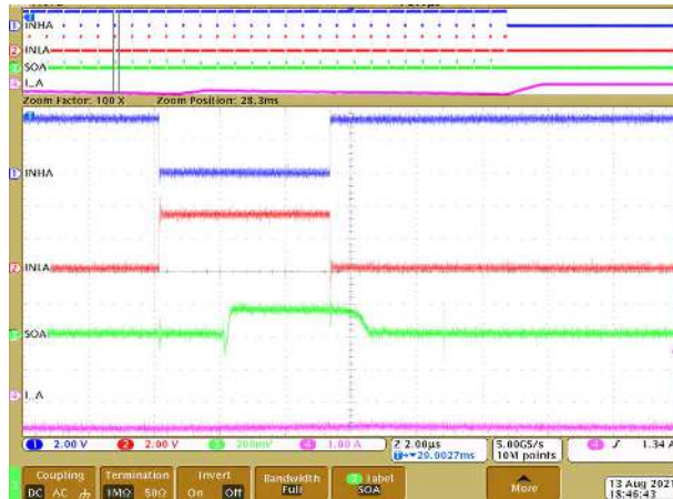
Figure 9-6. Driver PWM operation with feedback
