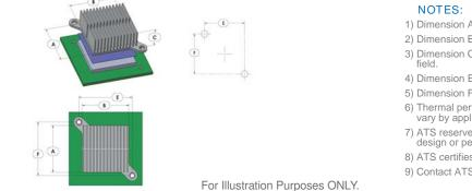
1) Dimension A is the length of the heat sink in the direction of the flow.
