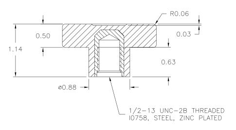
2830BG 2890-2830 CAVITY 2830 PLUNGER 2830 CAVITY PLUG 2830BG PLUNGER PIN 2830 INNER PIN 3000-J3 OUTER PIN 3000-J LANDING BAR .472 PIN PLATE SHIM .373 SHIM .018 INSERT 10758
