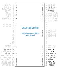
**Universal Socket Connectivity.** Multi-Tech's Universal Socket is a flexible, comm-port architecture that provides cellular, Ethernet, PSTN or Wi-Fi network access with interchangeable communications devices. This means you can utilize one system design and populate it with your connectivity device of choice accommodating multiple connectivity requirements. In addition, you are assured a seamless migration to future technologies.
