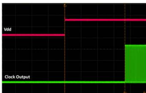
Figure 17. Startup Waveform vs. Vdd
