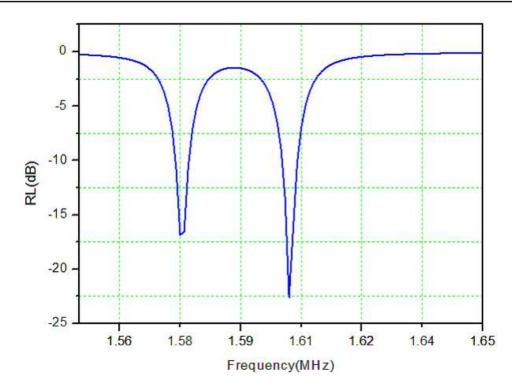
Return Loss characteristic shows a dual band response for GPS/Galileo & GLONASS R.H.).
