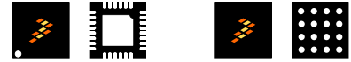
32-pin QFN (FM) 5 x 5 x 0.58 Pitch 0.5 mm 36-pin WLCSP (AL) 3.1 x 3.0 x 0.6 Pitch 0.4 mm
