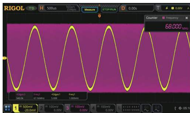
Observe and accurately measure two signals with great frequency deviations. The full-memory hardware measurement can measure accurate frequency value of the waveforms with 340k rising edges.
