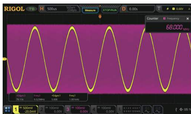
The ordinary 1 Mpts software measurement can no longer measure the accurate frequency of the high-frequency signal.
