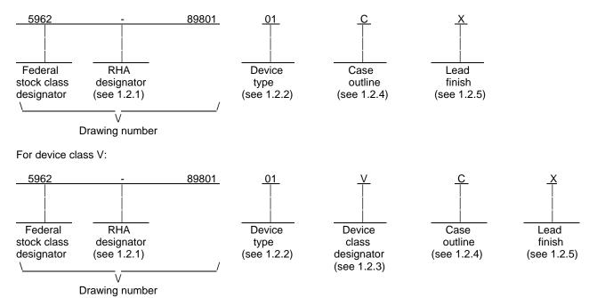
1.2.1 <u>RHA designator</u>. Device classes Q and V RHA marked devices meet the MIL-PRF-38535 specified RHA levels and are marked with the appropriate RHA designator. Device class M RHA marked devices meet the MIL-PRF-38535, appendix A specified RHA levels and are marked with the appropriate RHA designator. A dash (-) indicates a non-RHA device.
