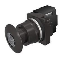
30mm BlackMax, Epoxy Coated Corrosion Resistant Complete Metal Unit Illuminated Push-Pull Operator Transformer type, 600V AC Incandescent Lamp Mushroom Head Cap Small 1 3/4" (44.5 mm) Metal, Black with Clear Lens 2 Position Maintained, Pull-to-Release UL Listed, CSA Certified NEMA 1,3,3R,4,4X,12,13 & Automotive Standards
