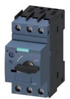
Circuit breaker size S00 for motor protection, CLASS 10 A-release 3.5...5 A N release 65 A screw terminal Standard switching capacity Multi-unit packaging Pack = 24 units
