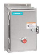
Non-reversing motor starter, Size 2 1/2, Three phase full voltage, Solid-state overload relay, OLR amp range 25-100A, Non-combination type, Encl. type 4X 304 S. Steel, Water/dust tight noncorrosive, Standard width enclosure
