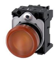
Indicator lights, 22 mm, round, metal, shiny, amber, lens, smooth, with holder, LED module with integrated LED 24 V AC/DC, screw terminal
