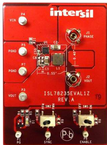
FIGURE 1. ISL78235EVAL1Z EVALUATION BOARD PHOTO
