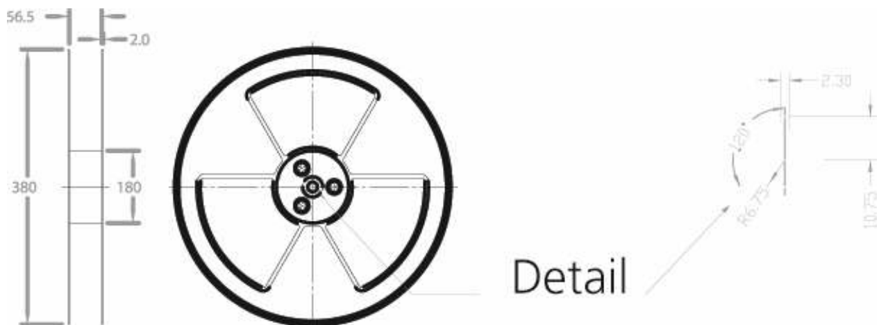
Figure 10: Dimension of reel for 250 pieces (dimensions in mm)
