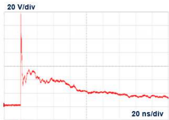
Figure 7. ESD response to ISO 10605 - C = 150 pF, R = 330 Ω (+8 kV contact discharge)
