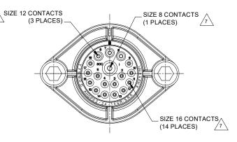
REDUCED DIA. WIRE SEAL SEALED PANEL MOUNT
