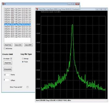
It can display trace files, and can back up and manage set-up files and other parameters into project folders.
