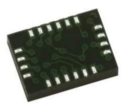
The HMC6042 utilizes Honeywell's Anisotropic Magnetoresistive (AMR) technology that provides advantages over other magnetic sensor technologies. The sensors feature precision in-axis sensitivity and linearity, solid-state construction with very low cross-axis sensitivity designed to measure both direction and magnitude of Earth's magnetic fields, from tens of micro-gauss to 6 gauss. Honeywell's Magnetic Sensors are among the most sensitive and reliable low-field sensors in the industry.
