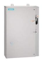
Non-reversing motor starter, Size 4, Three phase full voltage, Solid-state overload relay, OLR amp range 50-200A, 240V 50Hz / 277V 60Hz coil, Combination type, 200A fusible disconnect, 200A/250V fuse clip, Encl NEMA type 4X 304 S-Steel, Water/dust tight noncorrosive, Standard width enclosure
