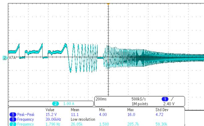
Figure 19. Motor Hitting Current Limit and Trying Again
