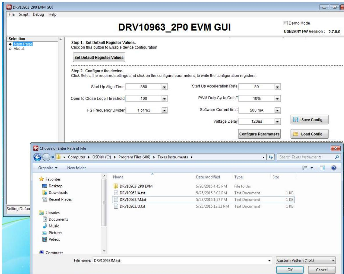
Figure 7. Loading DRV10963JM Configuration Parameter to Device
