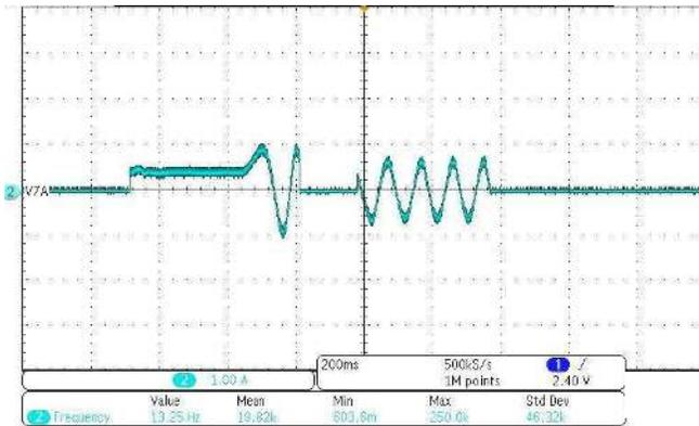
Figure 14. Open to Close Loop Threshold Too Low
