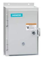
Non-reversing motor starter, Size 1, Three phase full voltage, Solid-state overload relay, OLRelay amp range 10-40a, 240V 50HZ / 277V 60HZ coil, Non-combination type, Enclosure type 12, Dust/drip proof for indoors, Extra-wide enclosure
