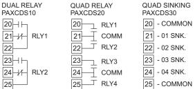
QUAD SOURCING/SSR DRIVE DUAL TRIAC/DUAL SSR DRIVE PAXCDS40 PAXCDS50 - EXTERNAL SUPPLY TRIAC 1 - 01 SRC. COMM 1/2 22 - 02 SRC. TRIAC 2 23 - 03 SRC. 23 - 03 SSR - 04 SRC. - 04 SSR - COMMON - COMM 3/4
