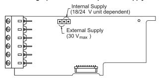
For Quad Sourcing/SSR Drive Option Card (PAXCDS40), set the jumper for internal or external supply operation before applying power.
