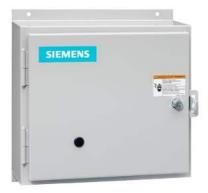
Non-reversing NEMA contactor, Size 1, Three phase full voltage, Contactor amp rating 27A, 3 wire (NO aux included), 110-120/220-240VAC 60Hz coil, Non-combination type, Enclosure NEMA type 12, Dust/drip proof for indoors, Standard width enclosure
