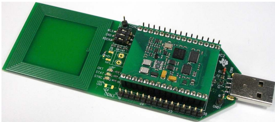
Figure 1. RI-STU-MRD2 EVM Board
