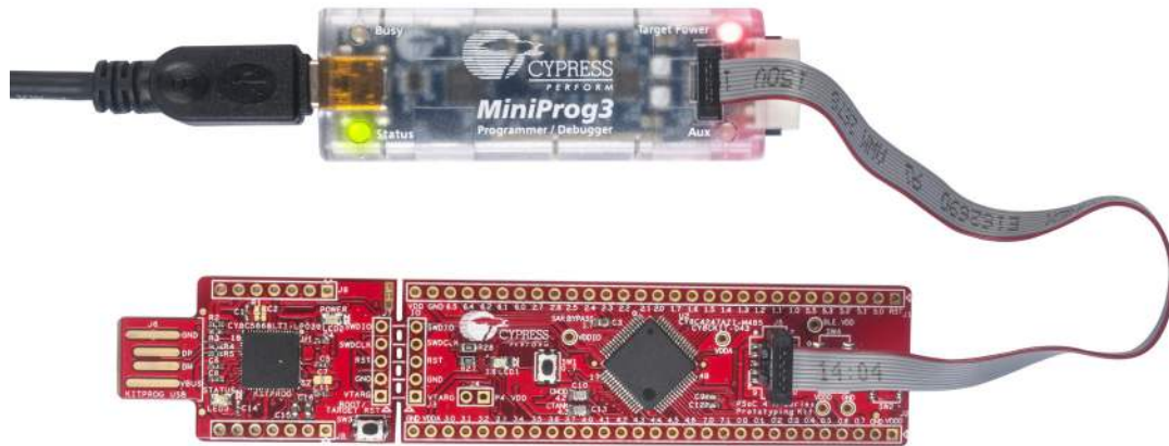
Figure A-1. Connecting CY8CKIT-043 to MiniProg3
