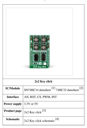
**2x2 Key click** has a 4 PCB button keypad. It carries the SN74HC14 Hex Schmitt-Trigger Inverter from Texas Instruments and 74HC32 quad 2-input OR gate from NXP. The click allows multiple key presses and is designed to use either 3.3V or 5V power supply.
