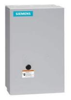
Non-reversing NEMA contactor, Size 0, Three phase full voltage, Contactor amp rating 18A, 3 wire (NO aux included), 220-240/440-480VAC 60Hz coil, Non-combination type, Enclosure NEMA type 1, Indoor general purpose use, Extra-wide enclosure
