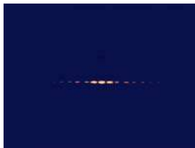
Figure 6. Laser diffraction pattern from dual slit.
