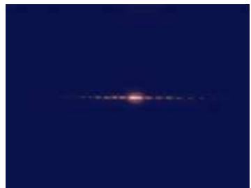
Figure 5. Diffraction pattern created by two razor blades.
