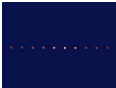
Figure 7. Optical beam pattern from the laser beam and the multiple slit array.
