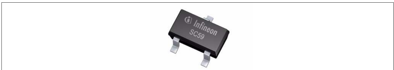
Figure 1 TLE4964-3K in the PG-SC59-3-5 package
