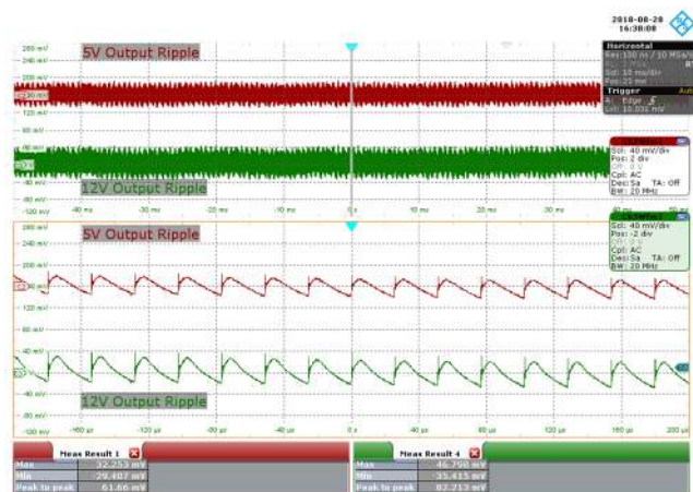
Figure 119 – 115 VAC 60 Hz, 50% Load. CH2: 5 V_{OUT} , 40 mV / div., 10 ms / div. CH3: 12 V_{OUT} , 40 mV / div., 10 ms / div. Zoom: 40 \mu s / div. 5 V Output Ripple = 63.241 mV. 12 V Output Ripple = 83.794 mV.
