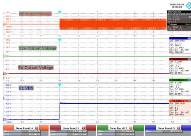
Figure 105 – Line Overvoltage during Normal Running Operation from 85 VAC. CH1: U1 V DS , 100 V / div., 1 s / div. CH2: 5 V OUT , 2 V / div., 1 s / div. CH3: 12 V OUT , 4 V / div., 1 s / div. CH4: AC IN , 200 V / div., 1 s / div.
