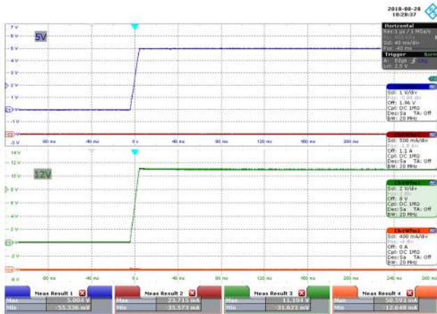
Figure 39 – 85 VAC 60 Hz, No-Load Start-up. CH1: 5 V OUT , 1 V / div., 40 ms / div. CH2: 5 V I LOAD , 500 mA / div., 40 ms / div. CH3: 12 V OUT , 2 V / div., 40 ms / div. CH4: 12 V I LOAD , 400 mA / div., 40 ms / div.
