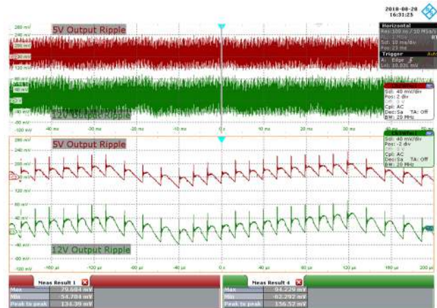
Figure 111 – 115 VAC 60 Hz, 100% Load. CH2: 5 V_{OUT} , 40 mV / div., 10 ms / div. CH3: 12 V_{OUT} , 40 mV / div., 10 ms / div. Zoom: 40 \mu s / div. 5 V Output Ripple = 134.39 mV. 12 V Output Ripple = 156.62 mV.
