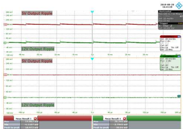
Figure 127 – 115 VAC 60 Hz, 0% Load. CH2: 5 V OUT , 40 mV / div., 10 ms / div. CH3: 12 V OUT , 40 mV / div., 10 ms / div. Zoom: 40 μs / div. 5 V Output Ripple = 17.391 mV. 12 V Output Ripple = 26.877 mV.
