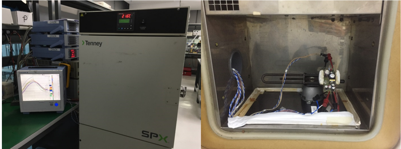
Figure 147 – Thermal Performance Set-up using Thermal Chamber.
