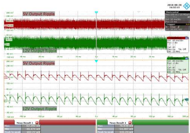
Figure 111 – 115 VAC 60 Hz, 100% Load. CH2: 5 V_{OUT} , 40 mV / div., 10 ms / div. CH3: 12 V_{OUT} , 40 mV / div., 10 ms / div. Zoom: 40 \mu s / div. 5 V Output Ripple = 134.39 mV. 12 V Output Ripple = 156.62 mV.
