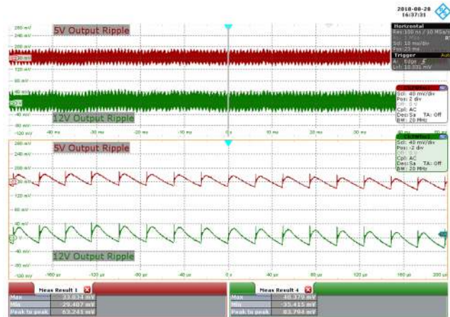
Figure 119 – 115 VAC 60 Hz, 50% Load. CH2: 5 V_{OUT} , 40 mV / div., 10 ms / div. CH3: 12 V_{OUT} , 40 mV / div., 10 ms / div. Zoom: 40 \mu s / div. 5 V Output Ripple = 63.241 mV. 12 V Output Ripple = 83.794 mV.
