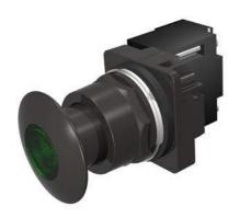
30mm BlackMax, Epoxy Coated Corrosion Resistant Complete Metal Unit Illuminated Push-Pull Operator Full Voltage, 12V AC/DC Incandescent Lamp Mushroom Head Cap Small 1 3/4" (44.5 mm) Metal, Black with Green Lens 3 Position Momentary UL Listed, CSA Certified NEMA 1,3,3R,4,4X,12,13 & Automotive Standards
