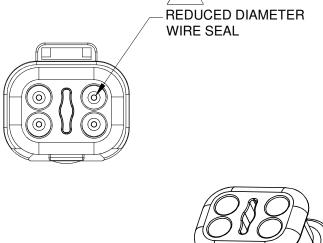
STRAIN RELIEF END CAP -BLACK - ALL — CONNECTORS RECEP, 4 PIN, AT, STRAIN RELIEF, REDUCED DIA WIRE SEAL
