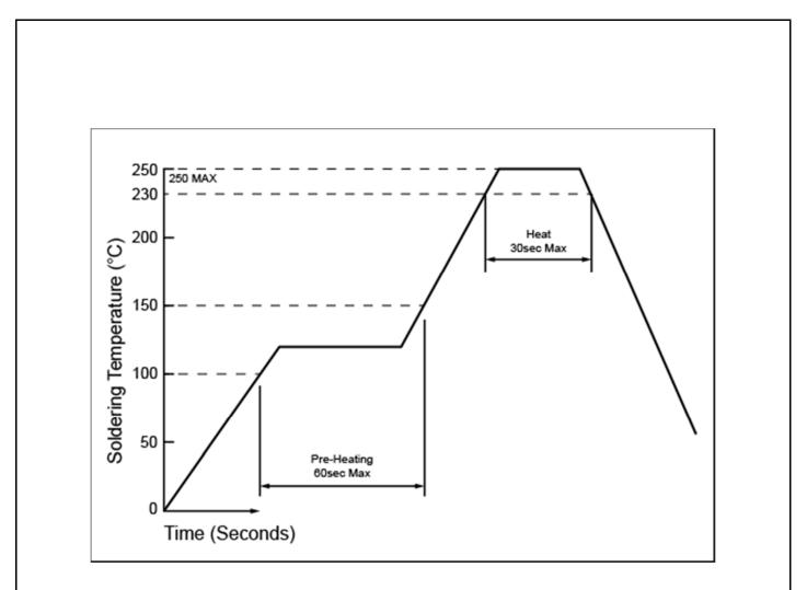
Fig. 1. Recommended Reflow Temp. Profile
