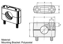
Hexagonal bolt and spring washer: Nickel-plated iron
