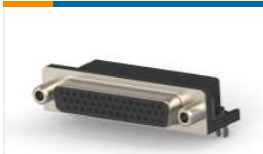
TE Part #2311770-1 AMPL REC, HD22, R/A, 44P, THREADED
