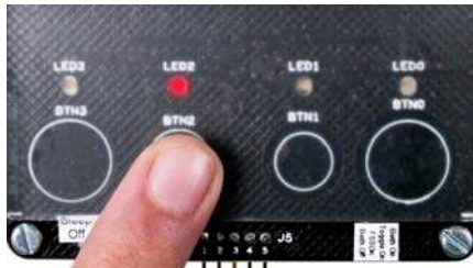
1. Touch a button; the LED turns on
