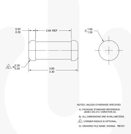
Figure 1. 2-TERMINAL, SOD-80, JEDEC DO-213AC, MINI-MELF
