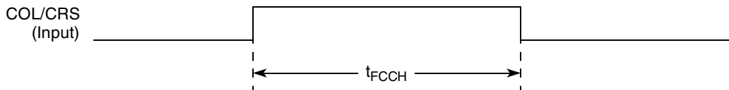
Figure 26. Ethernet Collision AC Timing Diagram (FCC)
