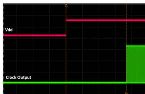
Figure 16. Startup Waveform vs. Vdd
