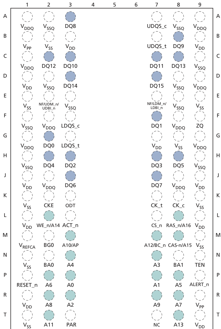
Figure 2: 96-Ball x16 Ball Assignments
