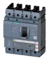
circuit breaker 3VA5 UL frame 250 breaking capacity class M 35kA @ 480 V 4-pole, line protection TM210, FTFM, In=100A overload protection Ir=100A fixed short-circuit protection Ii=10 x In N conductor protection 100% without connection
