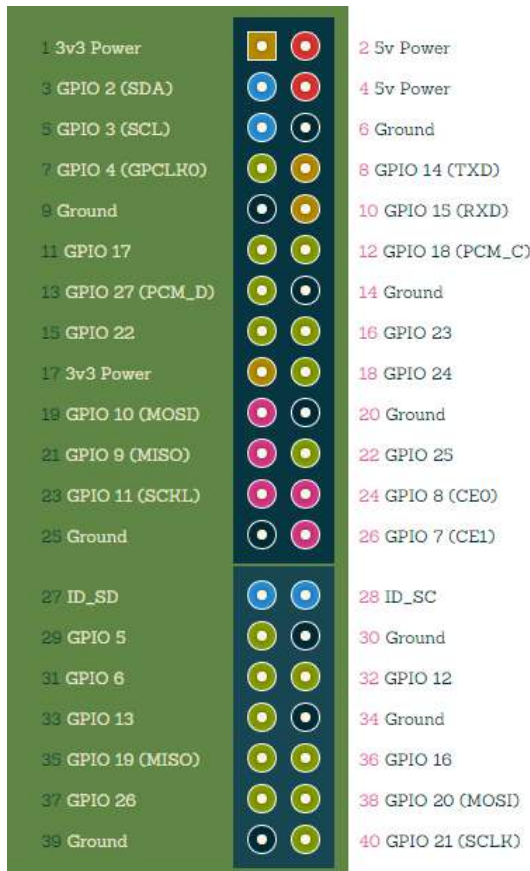
Raspberry Pi Pin Diagram
