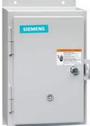
Non-reversing motor starter, Size 0, Three phase full voltage, Solid-state overload relay, OLRelay amp range 0.75-3.4a, 380 440/440 480V 50/60HZ coil, Non-combination type, Enclosure type 12, Dust/drip proof for indoors, Extra-wide enclosure
