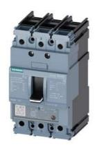
circuit breaker 3VA5 UL frame 125 breaking capacity class H 65kA @ 480 V 3-pole, line protection TM230, FTAM, In=30A overload protection Ir=30A fixed short-circuit protection Ii=5...10 x In cable connection on both sides
